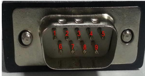
Fig 1-1 Male type interface (for RM060/120/200)
